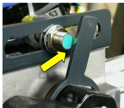
If required, loosen the nuts holding the switch, using the open-end wrench, and re-position the switch. Cycle the door engine to verify that the switches actuate and de-actuate properly.
