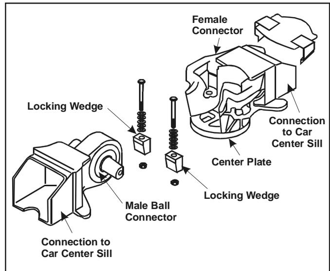
To separate the male and female connections, the locking wedges must be removed. **DO NOT** apply heat to any area of the ball connector to remove this unit. This could seriously affect the race of the ball connector.
