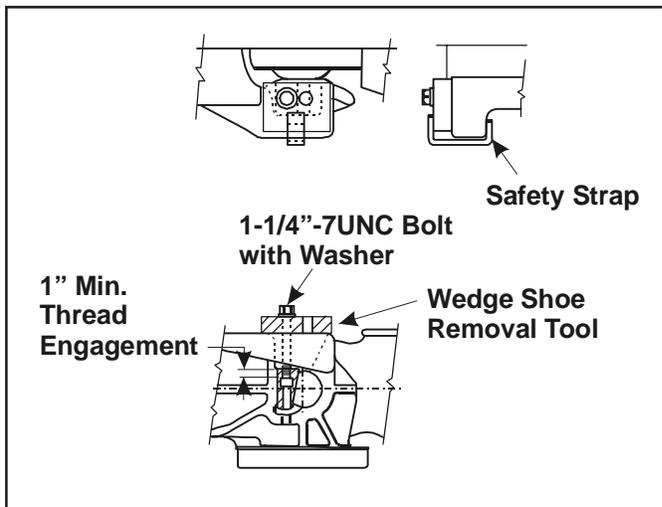
**WARNING:** *Extreme caution must be used when removing wedge, as it can become dislodged and eject at any time.*
