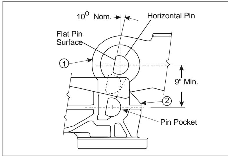
3. Install the two locking wedges (3) between the two flat pin surfaces of the male coupling (1) and the vertical machined surfaces of the female coupling (3). Match the vertical 90 degree surface of the locking wedge (3) with the 90 degree vertical machined surface of the female coupling (2), making sure to align the vertical hole in the locking wedge (3) with the drilled hole in the female coupling (2).
