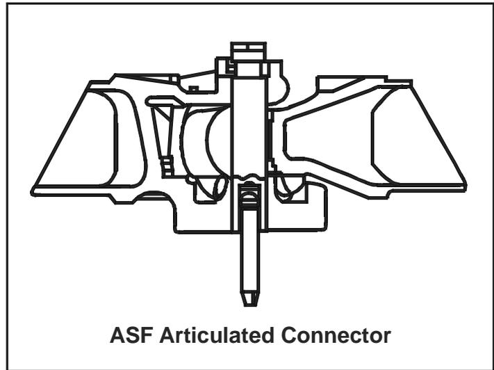
An important feature of the ASF connector is to make sure the wedge is all the way to the top before inserting the male connector. The wedge is held in place with a 1/2" rod, temporarily inserted into an opening in the casting on either side. Once the unit is connected remove the rod.
