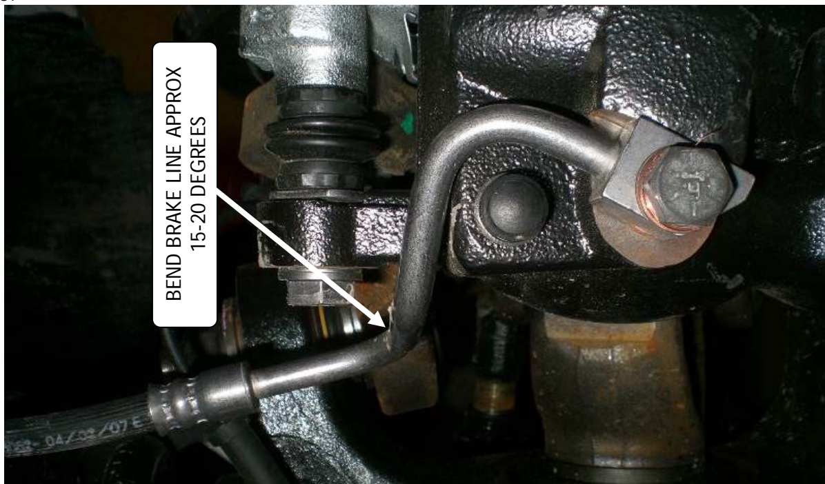
Figure 1 BRAKE LINE BENT AT APPROX. 15-20 DEGREES
