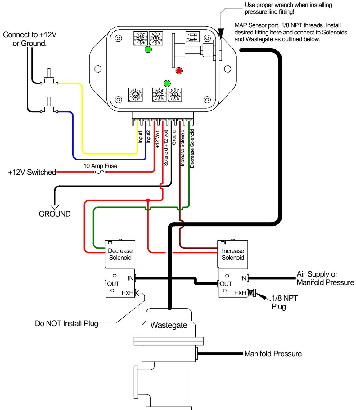
**IMPORTANT**—The AMS-500 controls the pressure on the Waste Gate so the actual boost level obtained is a combination of the Waste Gate Spring pressure and pressure applied by the controller
