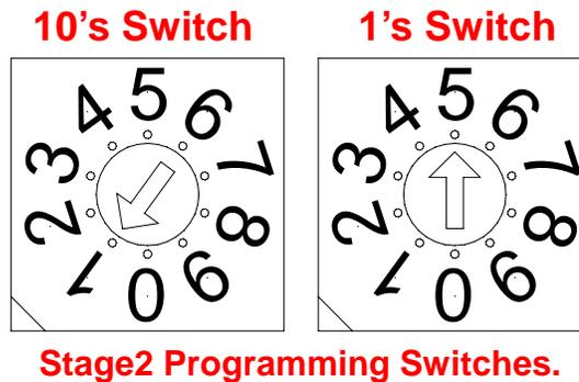
**Setting Stage2 Ramp Rate**—There are 16 Ramp Rates available for Stage2 boost control. These are selected using the Stage2 Ramp Rate Select Switch. A setting of 0 will result in the target pressure being applied immediately when Stage2 is active. See chart below for other Ramp Rates. The Ramp Rates are defined as psi per second.
