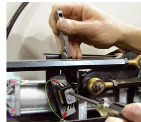
Use the feeler gauge to adjust for proper over-travel. Tighten the switch mounting screws. Cycle the door engine to verify that the switches actuate and de-actuate properly.
