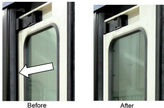
2. Check for proper closing by first opening the doors and then closing. Observe the leading edges when meeting at the center. Rear (#2) door panel should lead the front (#1) door panel when closing. If the rear (#2) door panel does not lead, lengthen the front door panel connecting rod until the rear door panel leads with no butting or touching as the edges overlap at the center.
