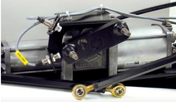
4. Close the rear (#2) door panel. While pushing the door panel closed, grasp the rear door spherical rod end (at the teeter plate) to prevent it from turning and turn the connecting rod until the rod end can slip onto the pin on the teeter plate. Install washer and lightly tighten nut.
