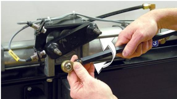
5. Close the front (#1) door panel. While pushing the door panel closed, grasp the front door spherical rod end to prevent it from turning and turn the connecting rod until the rod end can slip onto the pin on the teeter plate. Install washer and lightly tighten nut.
