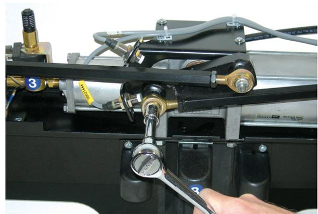
3. Make sure the connecting rods are clear of the teeter plate – **Keep Hands and Tools Away From All Moving Parts.** CLOSE the manual air valve – the teeter plate will move to the door closed position with the door controller set to the door closed position.
