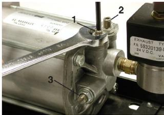
**Second: Adjust the opening speed.** Loosen the opening speed jam nut (2). Turn Allen screw clockwise to decrease opening speed – counterclockwise to increase speed. Disregard slamming against jamb. Tighten jam nut.
