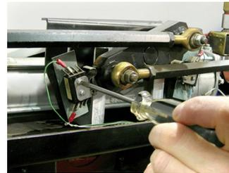
Proper adjustment must provide for a minimum of .015" of over-travel after actuation (over-travel is the movement allowed in the switch after actuation before the switch lever and plunger bottoms).
